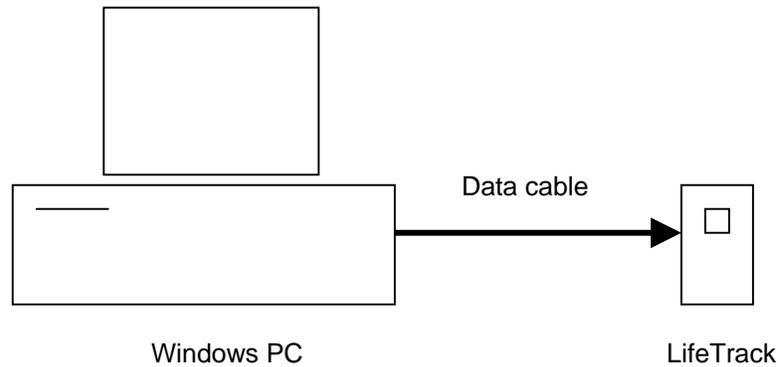
Before use, the LifeTrack units are subjected to additional QC testing and verification. To facilitate this process, the LifeTrack has the ability to operate in various "QC test" modes that test the unit at accelerated speeds, and report temperature sensor calibration by telemetry. These QC test modes enable large numbers of LifeTrack units to be calibrated, programmed, and tested using a high-volume, automated, manufacturing process.
